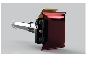
The heart of VPS-ROBERTA® is a servo-controlled robot arm which uses a specialized gripping technique to pick the desired products and transports them into a shopping cart.
